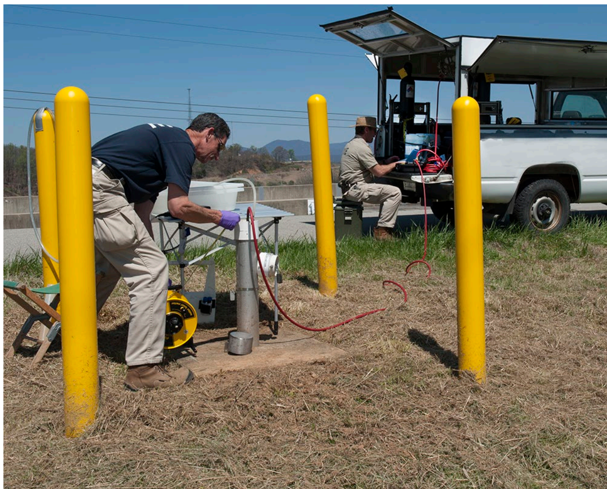
Figure 4.35. Groundwater monitoring well sampling at the Y-12 National Security Complex
